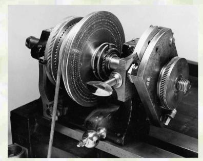
Figure 3102 Oval Chuck of the Holtzapffel Lathe of Otto von Habsburg, Vienna 1886 [1.1.3]
