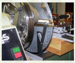
Figure 6309 Lee-Indexer ILI on the ovalturning Lathe ODM30, rear view (Workshop J. Volmer, Chemnitz 2007)
