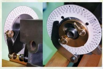
Figure 6304 Indexer for Ovalturning Lathe ODM15 (Workshop J. Volmer, Chemnitz 2001)
