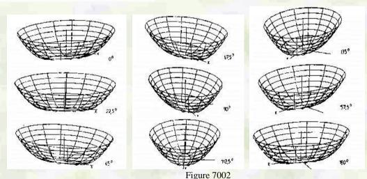
Perspective views of the bowl of figure 7001 in positions when rotating around its vertical z-axis
