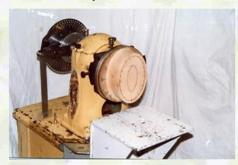
Figure 6303 Indexer ICI installed at the Myford Woodturning Lathe ML8 (Workshop E. W. Newton, Bradford 1994)
