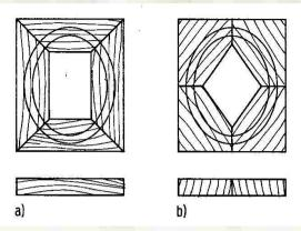
Figure 5402 Rectangle frame blanks a) Quarter-sawn b) Plain-sawn
