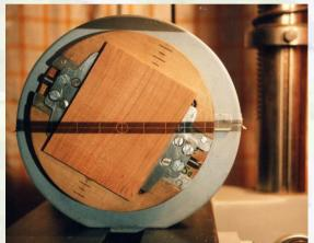
Figure 5404 Frame rectangle in the two-jaw chuck at the ODM15
