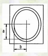
Figure 5403 Half-axes of the picture ellipse
