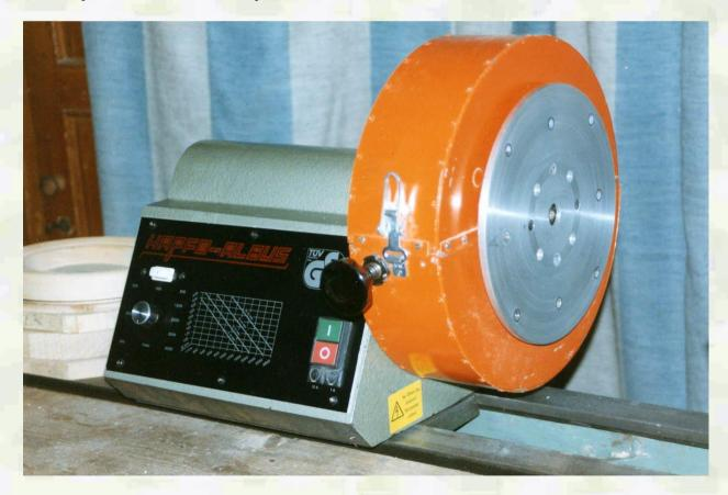
Figure 3403 Ovalturning Lathe ODM30 (Workshop J. Volmer, Chemnitz 1993)
