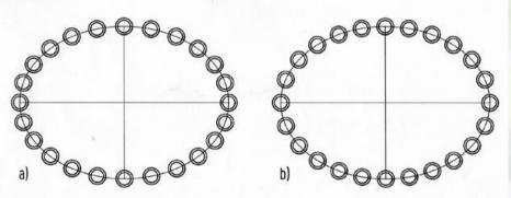
Figure 6103 Division of the ellipse in 24 parts a) by division plate: distances unequal
