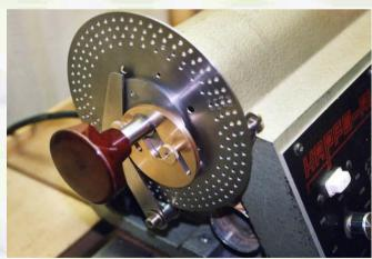
The Improved-Lee-Indexer (ILI) has the simplest of structures. It has been designed following an idea of Don Lee, in his time SOT-Member. The indexer consists of a normal division plate and a mechanism made of plain sheet metal parts, simple turned parts for joints and index pin (Figure 6308). There are instructions for its adjustment [2.2.17] [2.2.18]..
