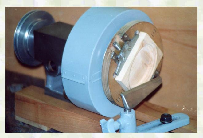
Figure 3402 Ovalturning Lathe (Ovaldrehmaschine) ODM15 (Workshop J. Volmer, Chemnitz 1989, photo Günther Göthl)
