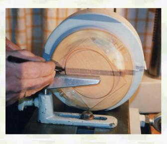
Figure 5406 Marking the picture-ellipse by the piercer
