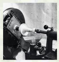
The possibilities of the design of shapes and profiles of objects turned using the ELLPIN device are endless. Some experimental candle-holders have been produced.
