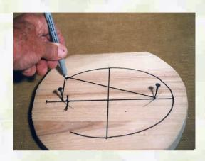
Figure 2102a Thread ring around three nails
