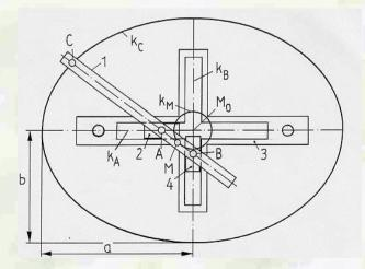
Figure 2103 Kinematic scheme of the Ellipsograph (trammel)
