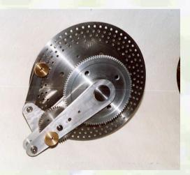
Holtzapffel [1.2.1] describes the "Compensating Index" as an Indexer. This ingenious but probably empirically dimensioned mechanism was invented around 1830. A kinematic analysis [1.2.5] has shown that this indexer could be substantially improved. Hence the "Improved Compensating Index" (ICI) has been constructed as indexer for the classic oval
