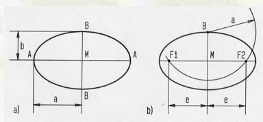
Figure 2101 Ellipse axes and linear eccentricity
