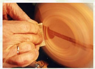
Figure 5408 Sanding the profile near the central line
