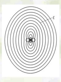
Figure 3202 Curves by an elliptical cam disk E
