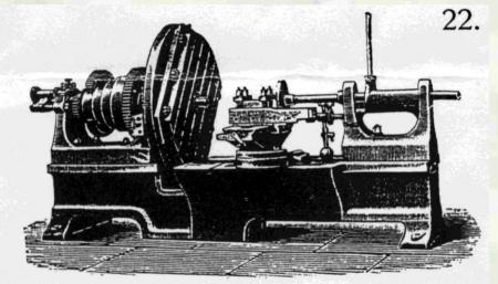
In Germany oval chucks (Ovalwerke) of the classic type were produced until 1950. These oval chucks were screwed onto the lathe as an additional device. There were also ovalturning lathes on the market built as single purpose machines. The principle of the classic oval chuck was also used on machines to form shallow oval bowls and plates from porcelain clay mass and also for spinning oval pieces on spinning lathes (Figure 3103).
