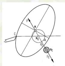
Figure 3305 Inertial forces of the ellipse motion of the classic oval chuck
