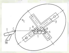
Figure 3301 Kinematic scheme of the oval chuck mechanism [5,5]
